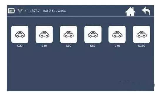
Before key programming Volvo XC60, you need to read the security data of two modules, then directly OBD add the key (add key and all keys lost are in the same way)
