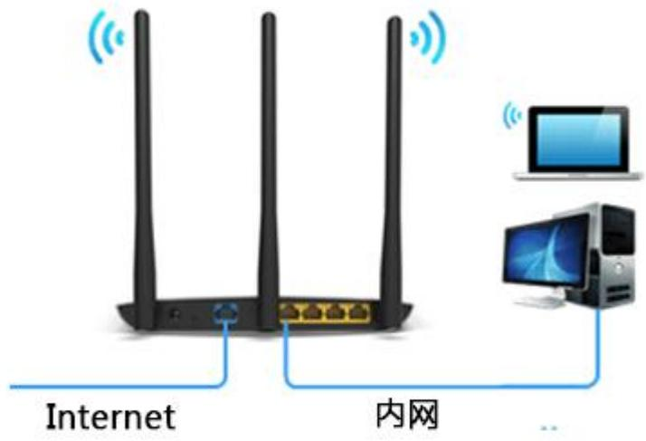
C. If there is NO WIFI access of the PC, please insert a WIFI adapter in the USB port and unplug the network wire of PC, then connect the same WIFI connected by cell phone.
