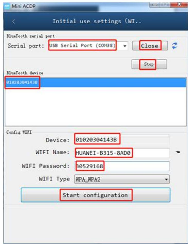
6.2: If the PC without WIFI access function, the PC is connected through a WIFI router with wired network. Follow the steps shown as below.
