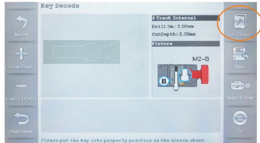
6) Select proper clamp, then click on 'Key Decode', probe will be detected many different points of whole key.
