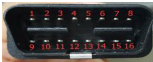
Pic 3: 16 pins on the vehicle OBD connector
